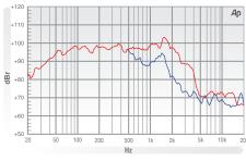
\* Half space response measured in a 975 litre sealed box
